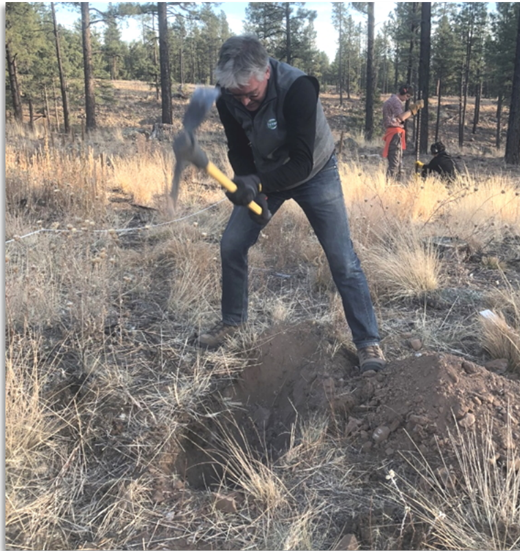
Figure 40. Willem van Leeuwen, Arizona Remote Sensing Center, digs a soil moisture sensor trench at a forest thinning site near Flagstaff, AZ. Snow stake installation in progress in the background. Photo: Joel Biederman.
