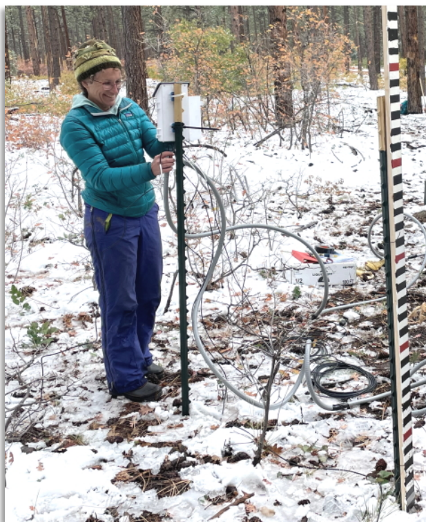
Figure 43. Gigi Richard, Fort Lewis College, configuring a soil moisture data logger at Chicken Creek, San Juan National Forest. Photo: Seth Arens.
