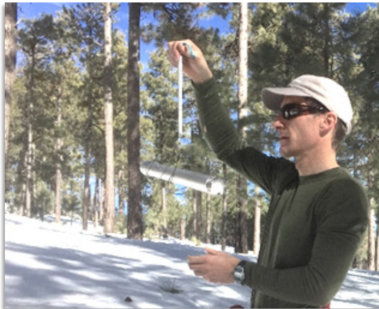
Figure 35. Joel Biederman weighing a snow tube for snow density measurement. A low-range spring scale is used for precise measurement in shallow snowpack. Coconino National Forest, AZ.
