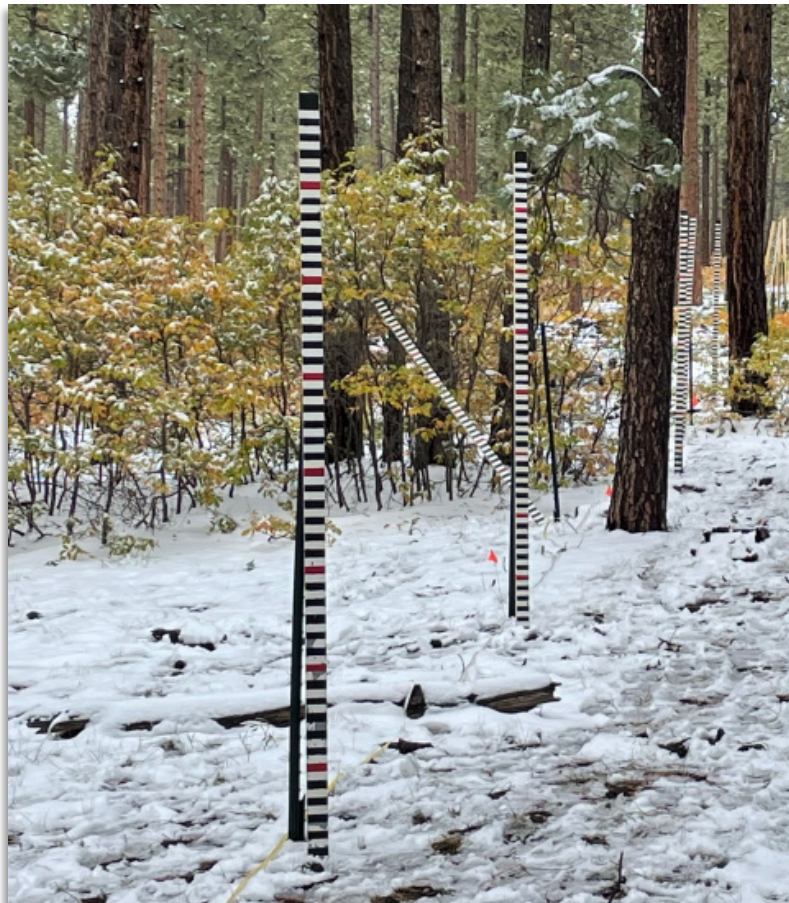
Figure 28. Snow stakes leaning on T-posts to check alignment with a snowtography camera. Photo also shows transect line (yellow tape) and stake locations (flags). San Juan National Forest. Photo: Seth Arens, Western Water Assessment.
