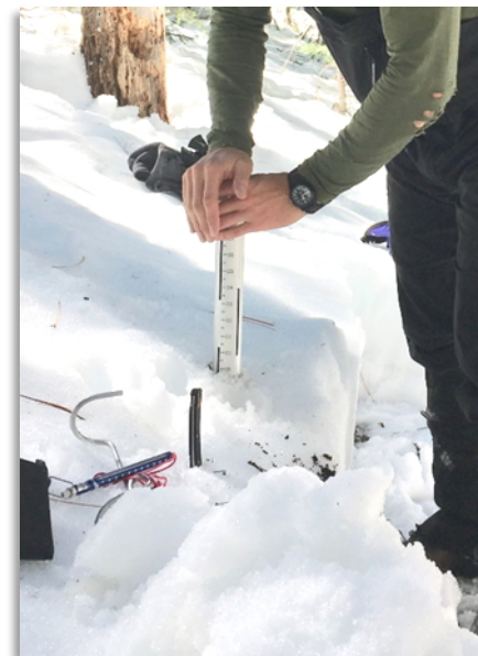
Figure 38. A federal sampler being twisted clockwise to engage the cutting teeth while being pressed through an ice layer within the snowpack. Photo: Patrick Broxton.
