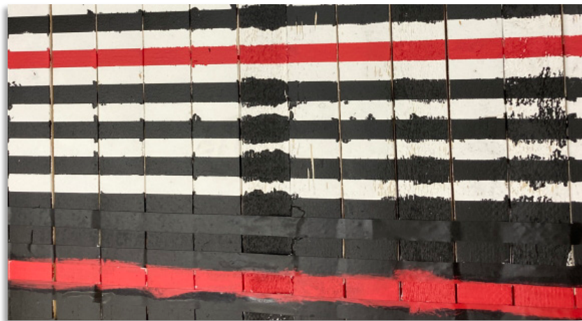
Figure 20. Photo showing how paint can bleed under the tape if a board is warped and the tape hasn't fully adhered. Photo: Lindy Hutchinson.
